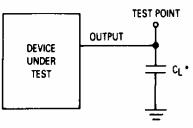
\*Includes all probe and jig capacitance.
