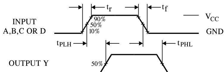
Figure 1. Switching Waveforms
