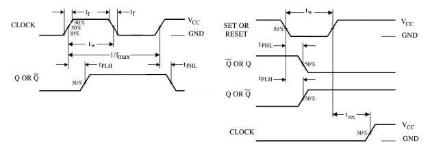
Figure 1. Switching Waveform
