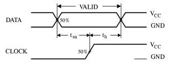
Figure 3. Switching Waveform
