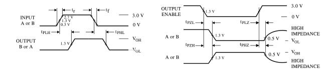
tpzl - S1 closed, S2 opened tpzh- S1 opened, S2 closed tplz, tphz - S1 and S2 closed
