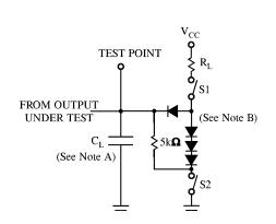
NOTES A. CL includes probe and jig capacitance. B. All diodes are 1N916 or 1N3064.
