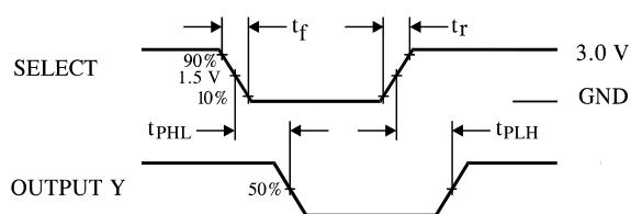
Figure 1. Switching Waveform
