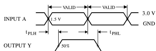
Figure 2. Switching Waveform
