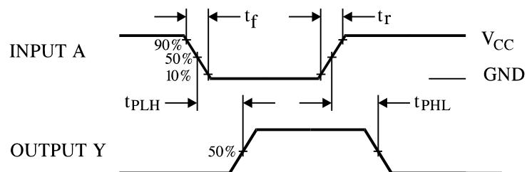
**Figure 1. Switching Waveforms**
